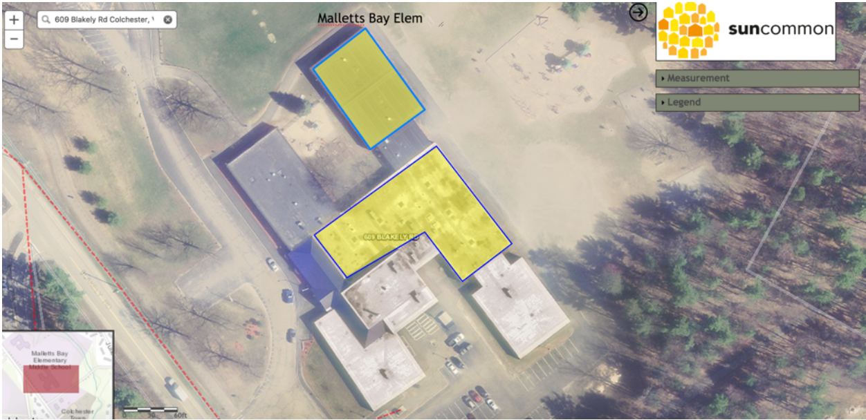
Malletts Bay Also has more than enough roof area for 150kWac (215kWdc) array.
